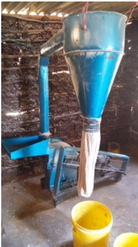
(Left) A posho (corn) mill powered by microgrid electricity in a Powerhive pilot village
